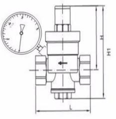
The use of direct action diaphragm structure, the internal structure is very simple, no jamming, reliable performance, durable.
